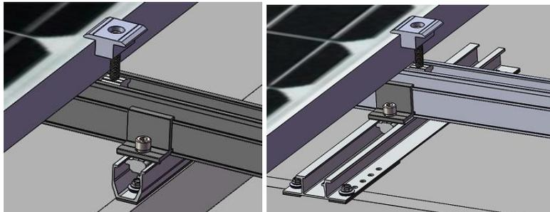
4.5.1.3 Loosely place the next framed PV Module into the other side of the Inter Clamp and as shown in Figures on the right.
