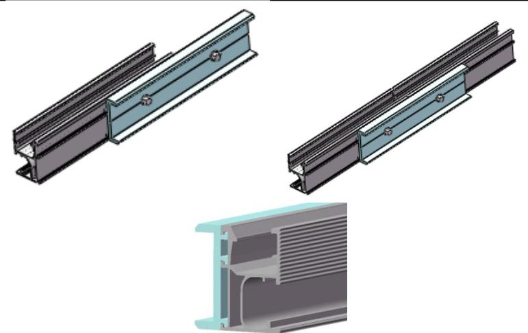
4.4.2 Place the ECO-Rail on the U support or Mycro Rail, uplift the Rail Clamp and click it into the side channels of the ECO-Rail as shown in the right figures. Fasten the Rail Clamp within 16-20 N.m torque after the Rail is positioned properly
