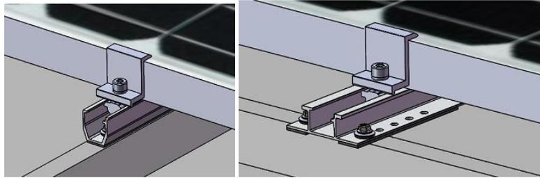
4.5.2.1 Repeat steps 4.5.1.2 and 4.5.1.3 to install the Inter clamp PV Module onto U support or Mycro Rail.
