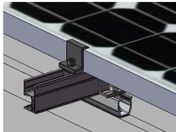
4.5.1.2 Click the Inter Clamp into the Rail and affix it to the side face of PV-Module. Don't fasten the bolt to make the installation of second PV Module easier.
